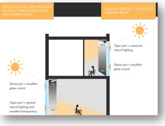
When the workspace is located near windows or when the glazing is of medium height, the open weaving of the fabric is positioned in the upper part of the blind to illuminate the room from the ceiling, while providing perfect glare control at the workstations.
